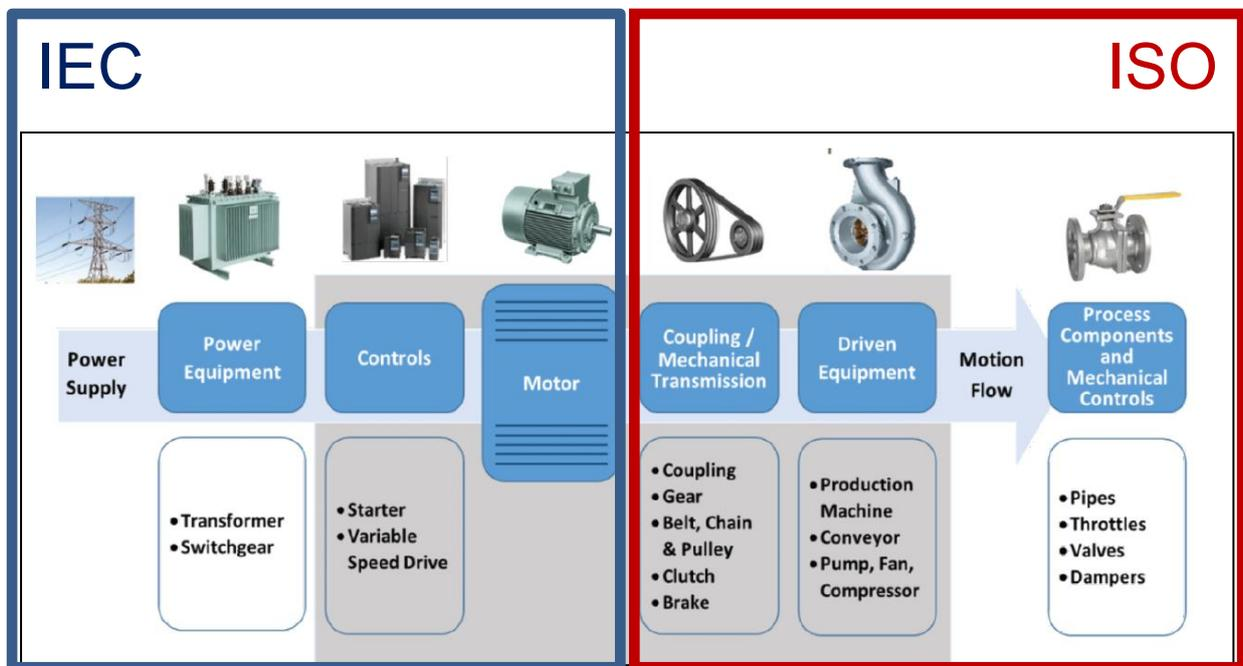
**Figure 1: The electric motor driven system and its major components**
