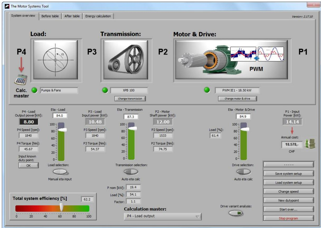
**Figure 6** The Motor Systems Tool (source: Danish Technological Institute, available at [www.motorsystems.org](http://www.motorsystems.org))
