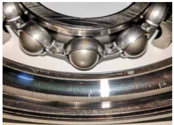
Photo: Ripple formation due to bearing currents (Source: Dr. Hanna Putzi-Plesko, ZHAW School of Engineering)
