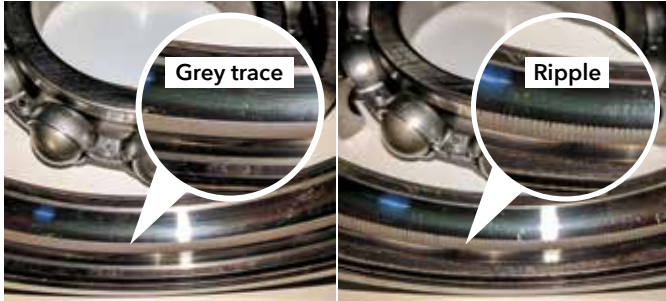
Figure 1: The two typical damage patterns caused by bearing currents; on the left: grey trace, on the right: ripple formation.
